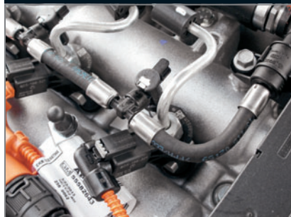
Like most clean diesels, the Cruze uses a common rail piezo injection system. That means high pressure and a need for common sense when servicing.
