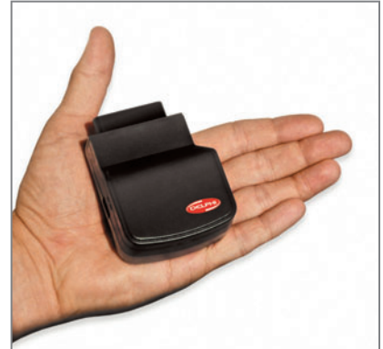
The Delphi unit connects to the DLC and provides a secure "car to cloud, cloud to car" connection.
