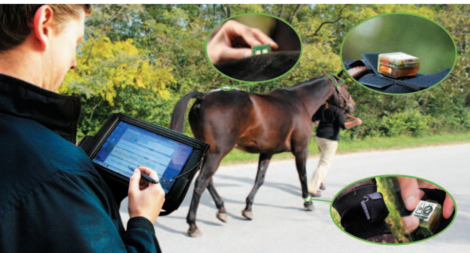
>>> An inertial sensor system (ISS; Lameness Locator—Equinosis) captures live motion data through wireless sensors for analysis.
