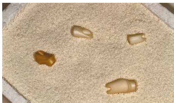
Fig. 5 Post pre-shading and sintering
