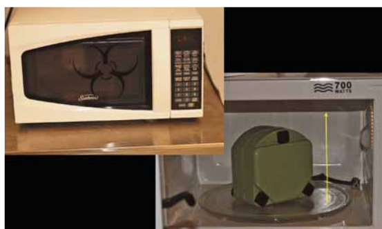
Fig. 6 Typical home use microwave ovens today have the features needed to deliver exact wattage and full exposure of waves to refine the way curing is accomplished. Technique refinements such as vertical placement on the turntable also help fulfill the promise of the chemistry available in resin technology.
