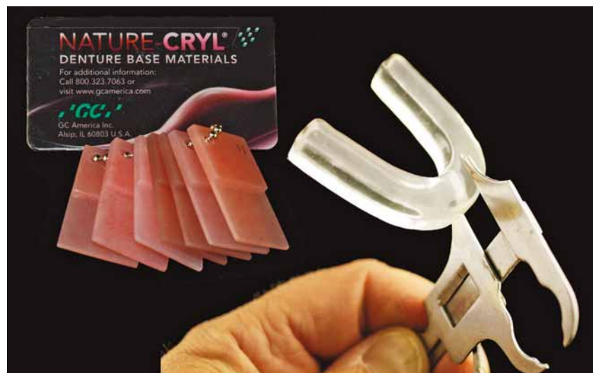
Fig. 4 Nature-Cryl MC is part of the GC America denture base line. Part of my research into the viability of using this product involved my testing of their microwave clear version. My rationale was if porosity or uncured areas existed after curing, it would be visible in the clear. The result was clear and porosity free, signaling to me that it had the performance I desired.
