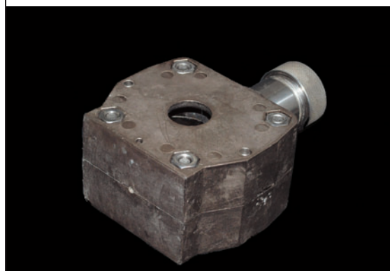
Fig. 8 Bolted injection flask necessitating a capping pour made through a hole in the top. Because you cannot see inside the flask, it is critical that the pour is smooth, flowing and bubble-free to provide a complete and accurate fill.
