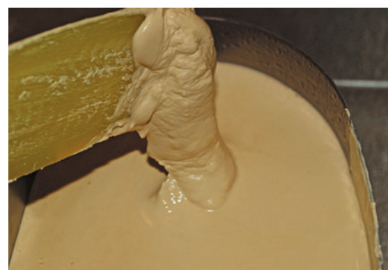
Figs. 7 and 7b Measurements for an average model are 150gr of stone to 50 mL of Wonderadmix. Consistency of stone when mixed for models or capping is smooth, creamy, and easy flowing. Slight vibration immediately causes it to flow.
