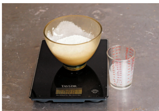
Figs. 7 and 7b Measurements for an average model are 150gr of stone to 50 mL of Wonderadmix. Consistency of stone when mixed for models or capping is smooth, creamy, and easy flowing. Slight vibration immediately causes it to flow.
