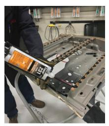
**NEW TECHNOLOGIES IN SOUND DAMPENING** allow some materials to be applied directly to bare metal. Direct-to-metal (DTM) technology resists surface corrosion while providing a sound-deadening solution.
