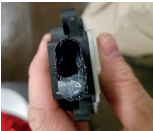
A CONNECTOR REPAIRED WITH RTV instead of using a new connector.
