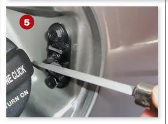
**4.** Use a triangular file to remove the required material from the top surface of each alignment guide, as shown. When filing is complete, use shop air to remove any debris from the fuel filler area.
