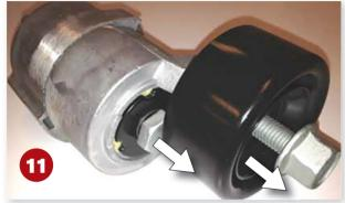
Torque pulley to the specification below: Tightening torque: 50 lb-ft (67Nm)
