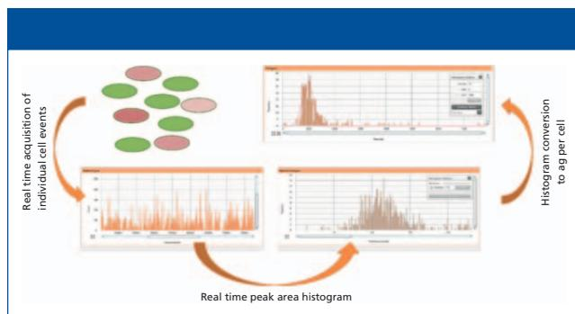
**Figure 3:** Conversion of metals within individual cells to mass per cell histogram using the Syngistix single-cell application software module.
