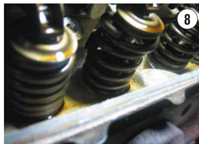
BROKEN EXHAUST VALVE SPRING ON 2005 GMC YUKON. This was found in less than five minutes of testing with a relative compression test after several days of testing and parts swapping by other technicians.
