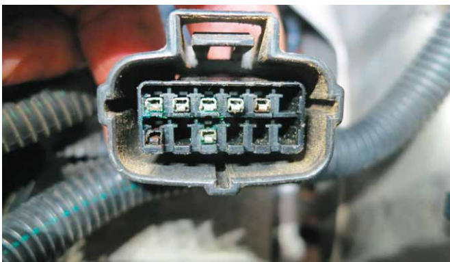
THE FREE-STAR'S TR SENSOR had a time-oxidized pin 12 — that was the reason for the stubbornly intermittent no-crank. There are pigtails and terminals to be had — at a cost. But that's the best fix for a problem like this.
