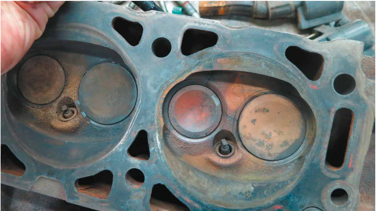
THE '99 MAZDA GOT HOT ENOUGH TO CRACK THIS HEAD , and a new one was in order. A few hundred dollars later, the B3000 was back on the road, at least until its next breakdown.
