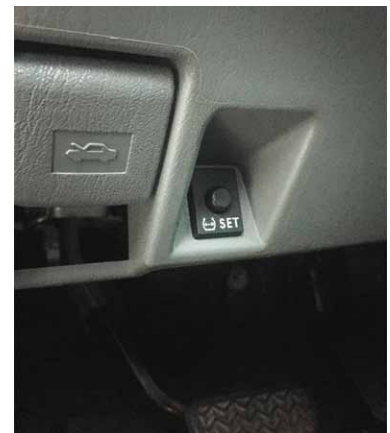
TOYOTA SET BUTTON FOR BASELINE TIRE PRESSURE
