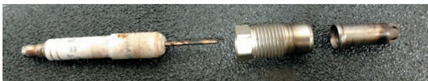
THIS IS A COMMON PROBLEM that occurs when trying to remove spark plugs on this type of engine. While the threaded portion separates from the cylinder head, the shell of the spark plug remains seized in the combustion chamber and special tooling is required to remove it.
