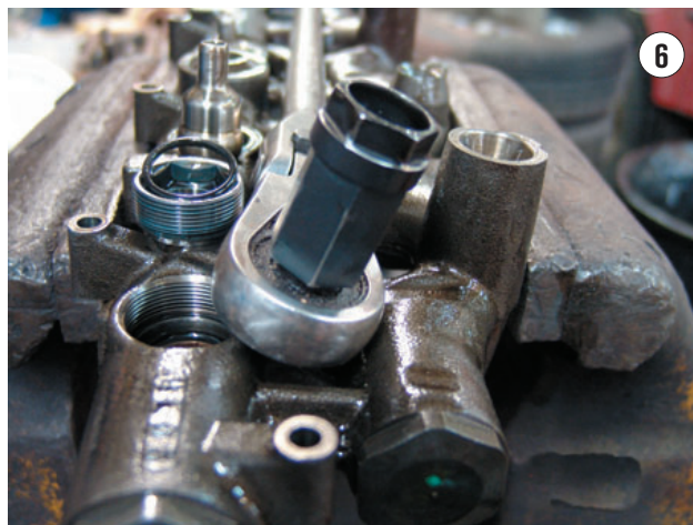
HIGH-PRESSURE OIL RAIL with one of the injector high-pressure oil nipples removed. These nipples have a seal under them that very commonly leak.
