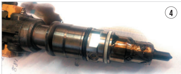
FUEL INJECTOR REMOVED FROM THE ENGINE. Notice the grease on the lower part of the injector. Injectors are supposed to be installed with motor oil to lubricate the seals. Using grease like this will plug up the fuel injectors.
