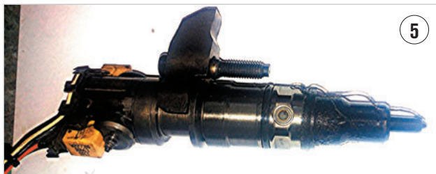
THIS FUEL INJECTOR WAS NOT PROPERLY INSTALLED IN THE ENGINE. Either the injector bore was not properly cleaned, or the injector hold down bolt was not properly torqued. Notice the black soot on the tip of the injector. This is caused by compression being blown up alongside the injector.
