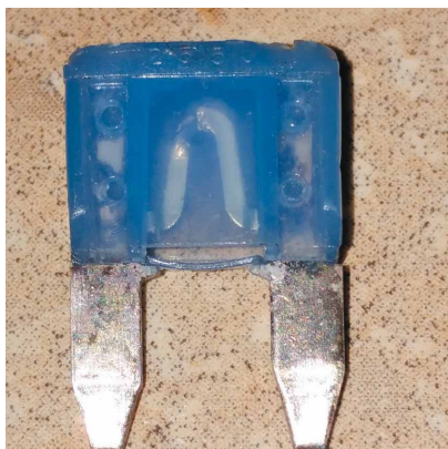
DAMAGED FUSE — loop broken from the "leg."
