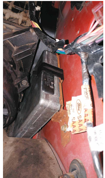
THE PCM IS MOUNTED inside the vehicle, on the right-side kick panel above and outboard of the blower motor.
