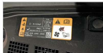
FORD CONTINUES TO BE THE ONLY OEM who lists the oil type and system charge amount along with refrigerant information on J639 underhood labels for all of their vehicles. This helps technicians know exactly which type of oil belongs in the system and more importantly, how much.
