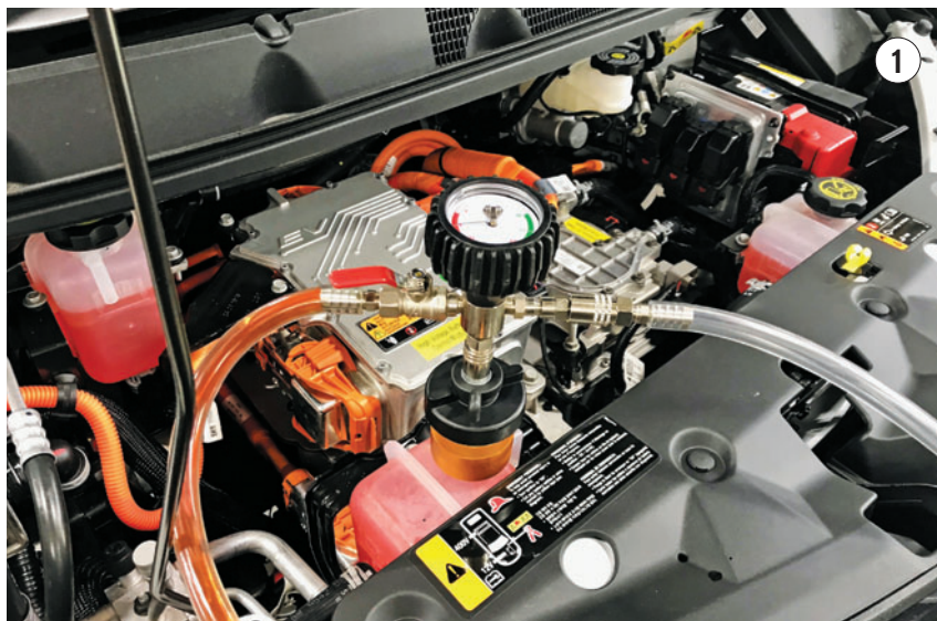
REFILLING THE HIGH-VOLTAGE BATTERY cooling system using a vacuum fill procedure on a 2017 Chevrolet Bolt EV.
