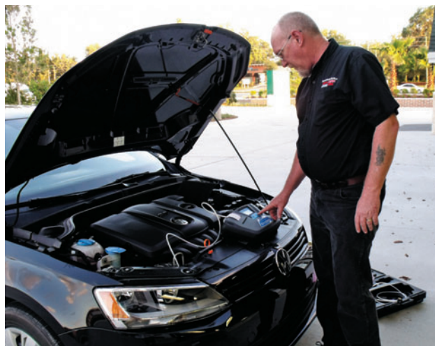
R1234YF MACHINES REQUIRE refrigerant identification prior to recovery and it's a "best practice" on any A/C system you service.
