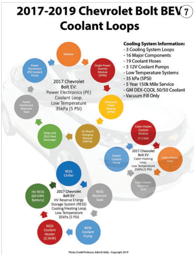
THE 3 COOLANT LOOPS of the 2016-2019 Chevrolet Bolt EV BEV
