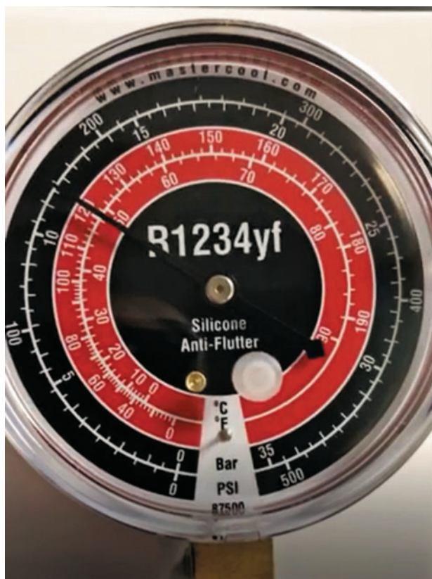
NORMAL HIGH-SIDE PRESSURE should hover around 175 psi. with everything working correctly. Photo courtesy of Dick Kreiger — ConsuLab product is EM-2000HB1234yf A/C trainer.
