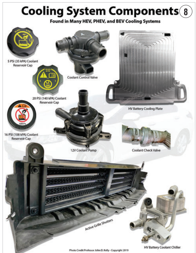
HEV, PHEV AND BEV cooling system components
