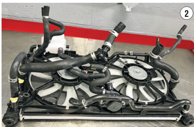
THE 2017 TOYOTA PRIUS has a two-section radiator, five cooling loops, 16 major components, 20 coolant hoses and two electric coolant pumps.
