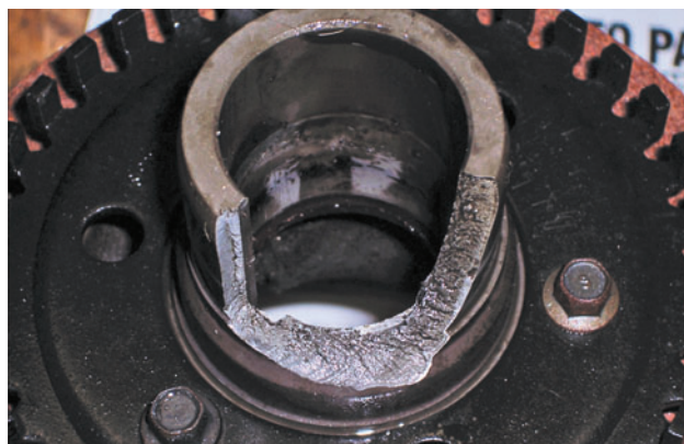
A BROKEN CRANKSHAFT BALANCER caused the CKP reluctor to shift.
