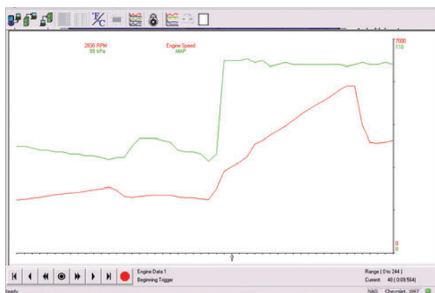
THIS IS HOW WE WANT a MAP sensor to react.
