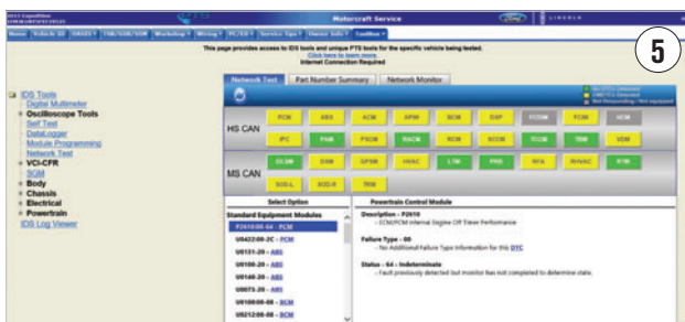
IDS SESSION STARTED by the Motorcraft/PTS website showing modules that have responded and those with DTCs in yellow.
