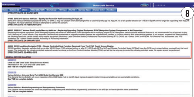
SSM, WHICH DESCRIBES that the climate seat function has been removed from the SYNCH touch screen
