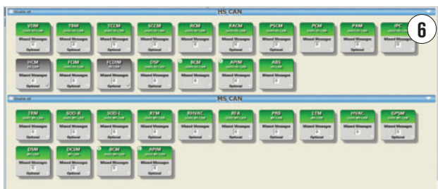
IDS SCREEN SHOWING interactive and live module testing. Gray shows modules that may be in the vehicle and are not responding. Green shows modules that are responding when pinged.
