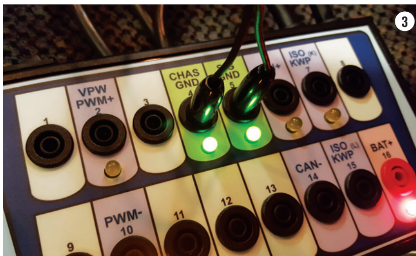
A JUMPER WIRE was used to provide a good ground to pin 5 of the DLC.
