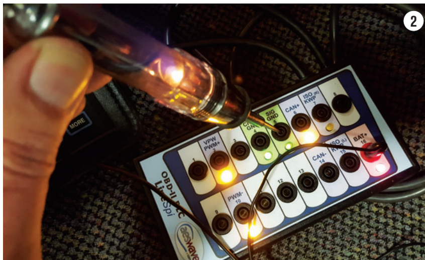
PIN 5 OF THE DLC has a voltage drop that can be seen due to the lack of test lamp intensity.
