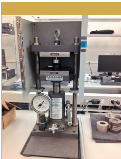
Figure 1: Typical sample press. There is a die between the platens and extra dies to the right of the press.
