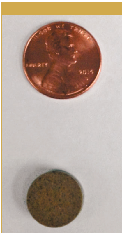
Figure 2: Pressed soil pellet ready for analysis.
