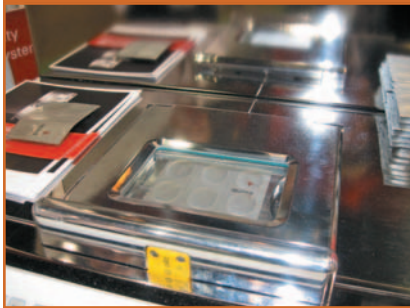
Figure 2: In a Pharma EXPO demonstration, the standalone AMI 120 leak detector from Pfeiffer Vacuum checked cold-formed foil blisters.
