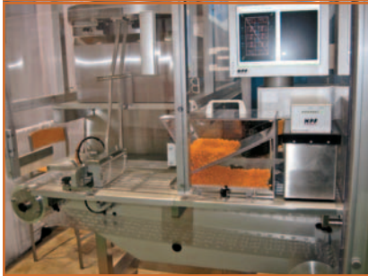
Figure 2: In a Pharma EXPO demonstration, the standalone AMI 120 leak detector from Pfeiffer Vacuum checked cold-formed foil blisters.
