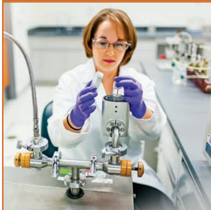
Figure 1: Helium leak testing is one way West Pharmaceutical Services checks container and closure integrity.
