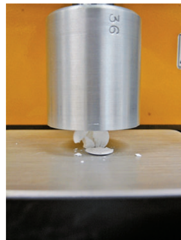
Figure 2: Cylinder probe fractures tablet in crush test (CT3 Analyzer, Brookfield Engineering).
