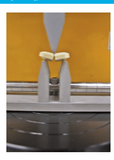
Figure 6: A blade splits the tablet in a bending test (CT3 Analyzer, Brookfield Engineering).
