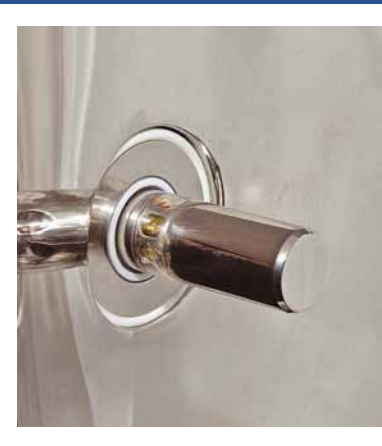
Figure 1: An in-process optical probe enables process analytical technology (Lighthouse Probe, GEA Pharma Systems).
