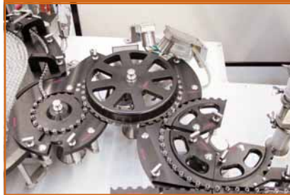
Figure 1: Groninger's aseptic vial-filling line offers contact-free container handling.
