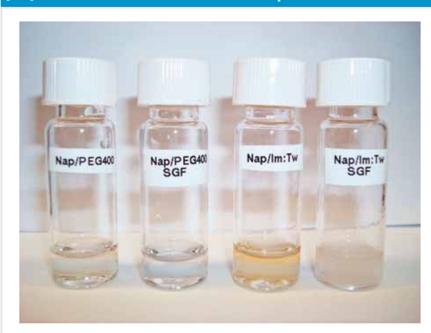
Figure 6: Naphthol/polyethylene glycol 400 (PEG 400) formulation before and after dispersion into simulated gastric fluid (SGF) and naphthol/Imwitor 742:Tween 80 [1:1] formulation before and after dispersion into SGF.
