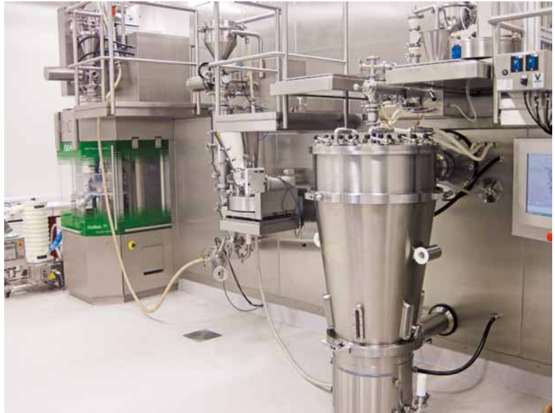
Figure 2: A continuous, high-shear granulation and drying system in operation at the GEA test center (ConsiGma, GEA Pharma Systems).
