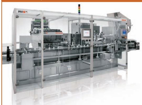
Figure 2: Monoblock machines, such as IMA's Uniline system, combine multiple functions on one base to enhance flexibility and reduce floor space requirements. Photo is courtesy of IMA.
