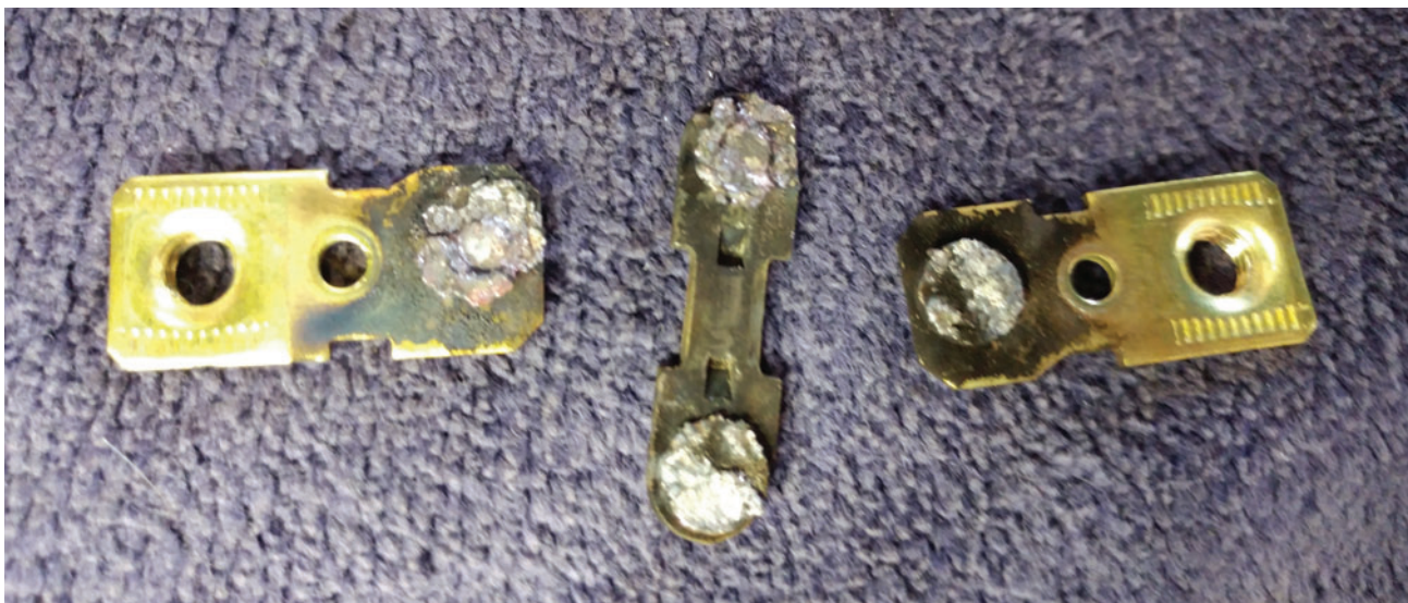
BURNED CONTACTS ON RESIDENTIAL HVAC UNIT - Once disassembled, it's obvious the electrical contacts could not conduct well, much like a starter solenoid's contact disk that is worn.
