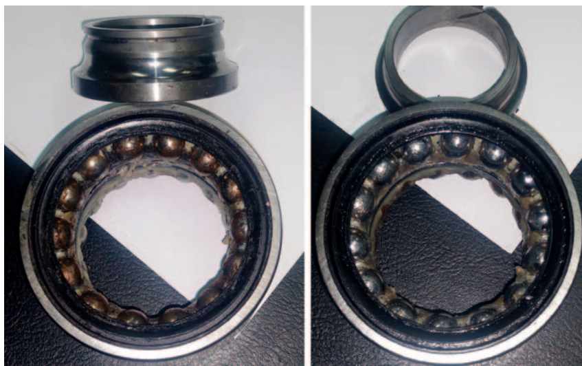
THE ONLY DIFFERENCE BETWEEN the noisy bearing and the non-noisy one was the color of the grease; there was no visible wear on the balls or the race.
