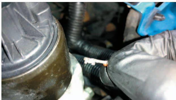
THE LOCKING TANG OF THE TERMINAL was bent and flattened, allowing it to back out of the connector and thus cause an intermittent circuit problem.
