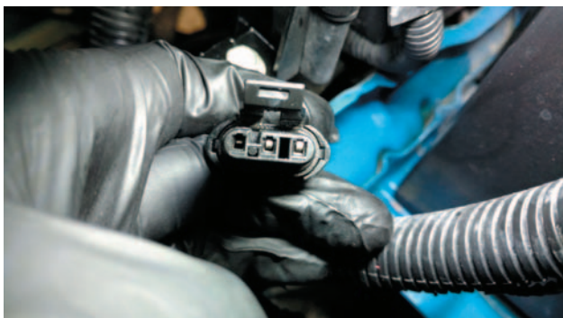
WHEN ATTEMPTING TO PERFORM A PIN DRAG TEST at the connector for the ignition module, the terminal pushed out of the back side of the connector.
