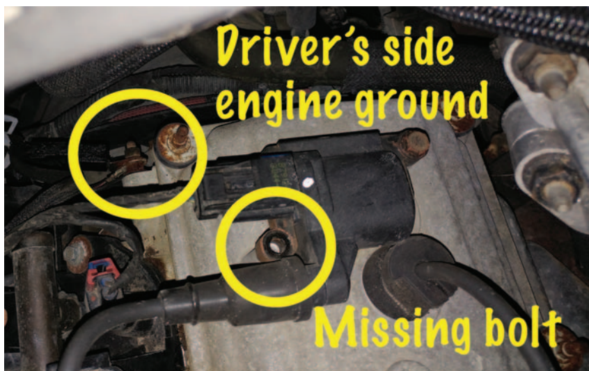
THERE IS ONE GROUND LOCATED on the rear of each cylinder head.
