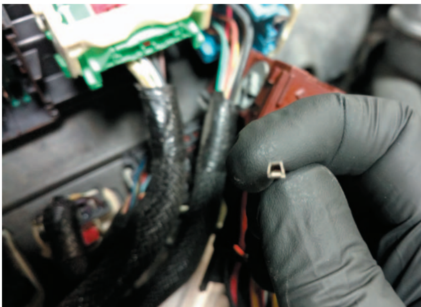
A CLOSE UP of the spread-open terminal connector causing a poor connection at the TIPM
