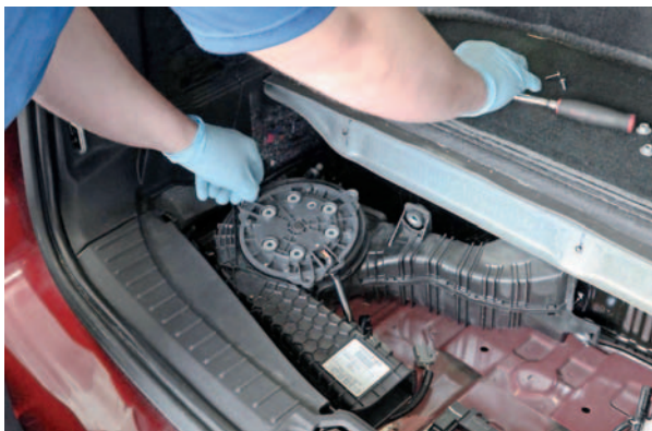
REPLACING THE HYBRID VEHICLE BATTERY COOLING FAN HELPS MAINTAIN OPTIMUM BATTERY LIFE.
