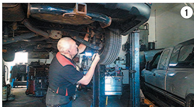
ALBIN MOORE USING HIS HANDS and a stethoscope to find a rough wheel bearing.
