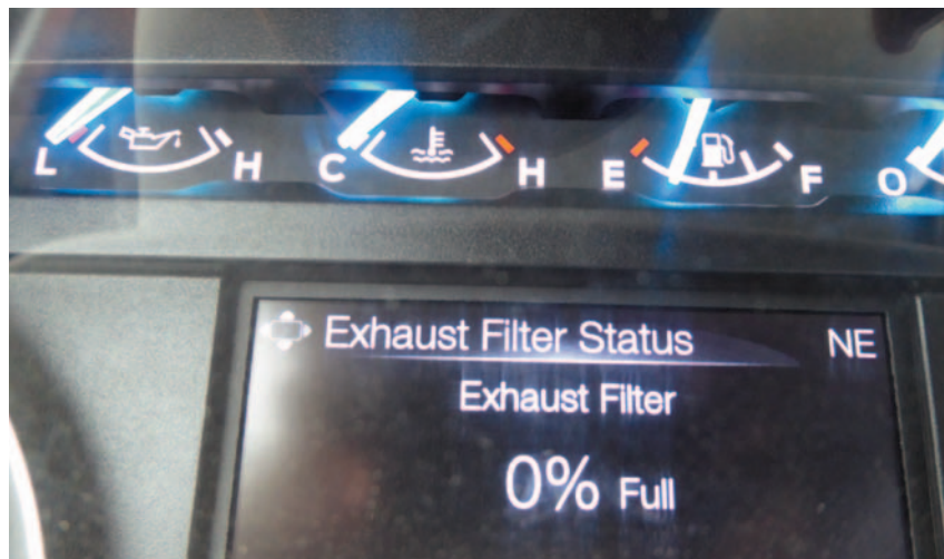
SCROLLING THROUGH THE INFORMATION SETTINGS on this Ford F-550 shows the diesel emission system monitors — helpful indeed.
