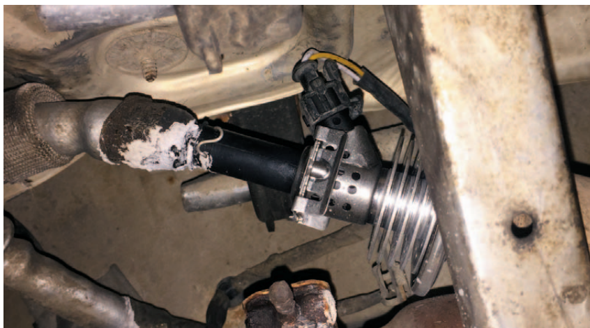
METERING VALVE - PRESSURE LINE LEAKAGE
