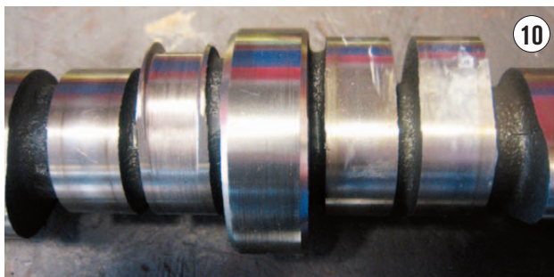
THE WORN EXHAUST CAM LOBE IS THE SECOND FROM THE LEFT IN THIS PICTURE.
