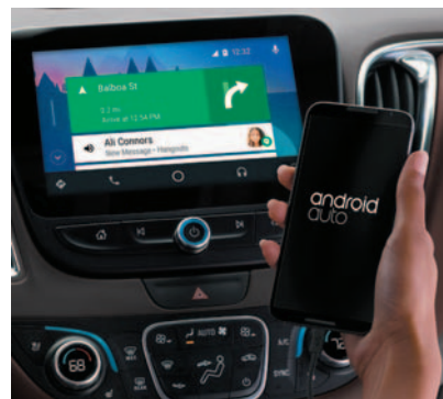
THE ANDROID AUTO APP INTERFACES with the vehicle's on-board display using the OEM steering wheel controls, touch screen and voice commands.
