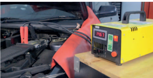
A CLEAN SUPPLY OF POWER IS ESSENTIAL to a successful flash, and that's something a typical shop battery charger can't deliver.
