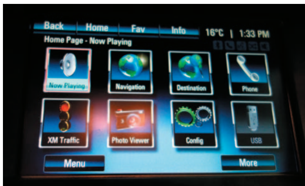
MOST STORED DATA AND SETTINGS CAN BE CLEARED or reset directly by navigating through the display screen and selecting the option something along the lines of "Settings," "Configurations," "Advanced" or "Options" — and then selecting the option to delete pairings or data stored, or even restoring the factory settings (which erases everything). The customer may still need to delete the pairings, permissions and apps from their phones or devices.
