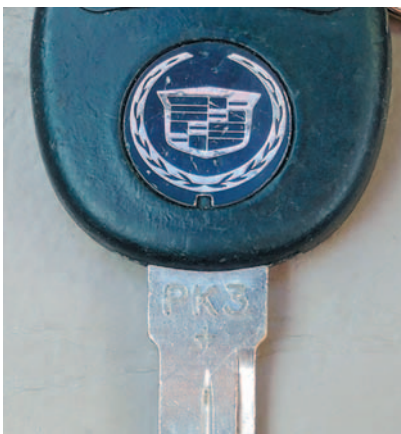
THE MASTER IGNITION KEY showing "PK3" stamped in the blade. Without the Master key, the VTD may not program correctly.
