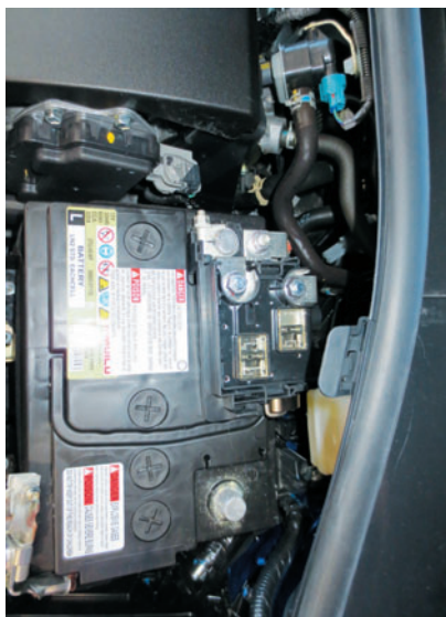
QUICKLY INSPECTING the condition of connections, fuses and fusible links can save headaches later on.
