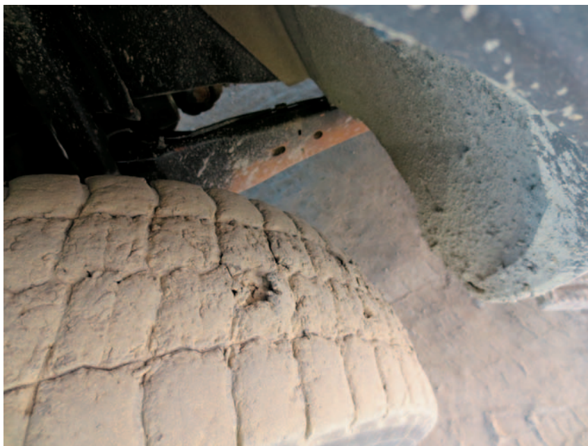
THIS TRUCK CAME IN WITH ITS TPMS LIGHT ON. A quick visual inspection found that in addition to the TPMS issue, it was also time for new tires — well past time, actually.
