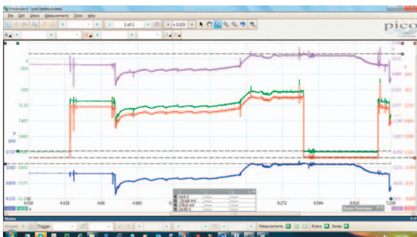
NOT ONLY DID THIS TEST prove a fault in the ignition switch, it also identified a weak battery.
