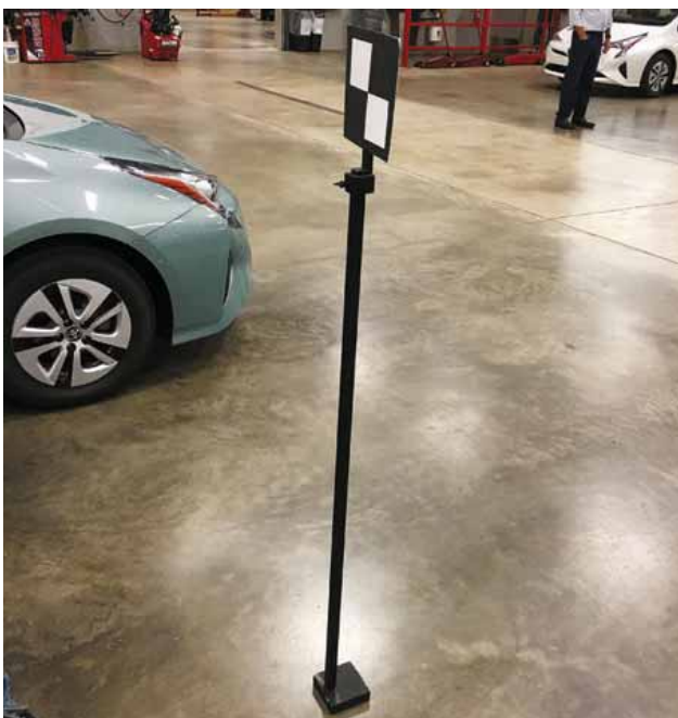
TOYOTA UTILIZES A SPECIAL SERVICE TOOL STAND and a target that can be printed from the service information to perform a calibration of the forward-facing camera.
