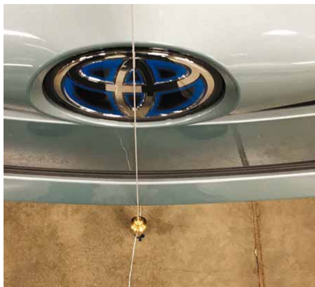
A PLUMB BOB is used to determine the center line of the vehicle.
