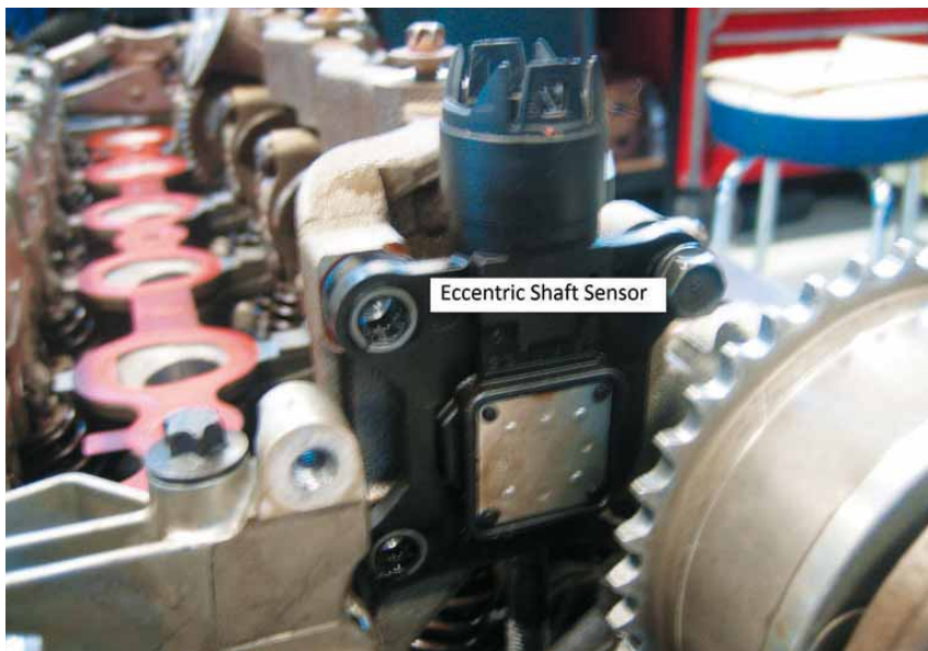
ECCENTRIC SHAFT mounted on N52 head with valve cover removed.
