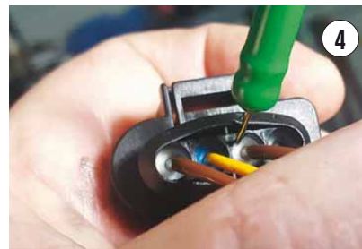
IT'S A BIT HARD TO SEE , but in this example the backprobe is on the outside of the weather seal – not good.
