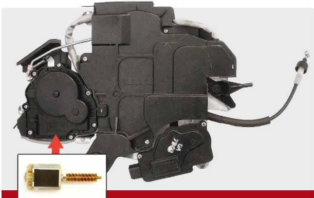
Power Sliding Door Remote Controller Assembly P/N 81447 4D500 Actuator Motor Shown Externally
