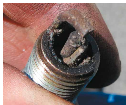
WE WON'T KNOW until later this summer what happened on the 2004 Suburban to cause this, but the cylinder it came from has almost no compression at all. And since the mileage is so high, we'll probably stuff an engine in it.
