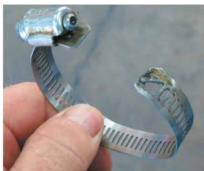
THIS IS ONE OF THOSE STEALTH PROBLEMS — one of my guys had replaced the radiator in this high mileage Ranger, and since the lower radiator hose clamp had seemed okay, he re-used it. What he couldn't see was that this clamp wasn't quite long enough; the screw was only holding a couple of slots, and they gave way one day about six weeks after the radiator was replaced and dumped the coolant.
