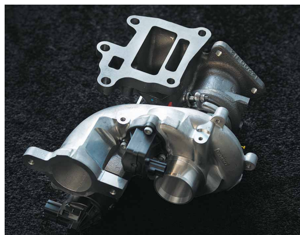
THE MAZDA Skyactiv-D Sports a two-stage turbo.
