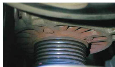
THIS TATTLETALE RUST STAIN was from a rattling alternator decoupler pulley on a Jeep Compass — the owner thought it was a bad A/C compressor and was pleasantly surprised at the easy fix.
