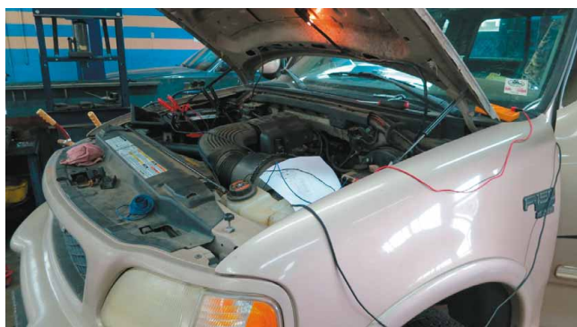
THIS '98 F-150 had a laundry list of issues — the least likely of which was the inoperative check engine light. We ran an overlay between the PCM connector and this bulkhead connector and got the light back online.
