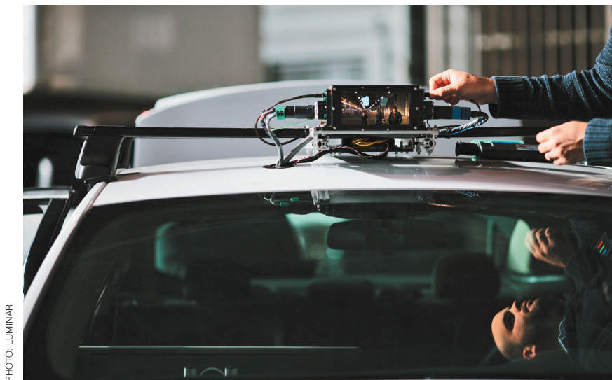
THIS LIDAR UNIT is manufactured by Luminar. The company is working on extending the range from its current 120 meters to 200 meters.
