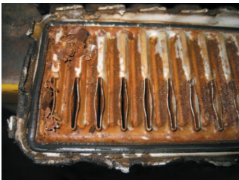
RUST ATTACKS PARTS FROM THE INSIDE OUT in a very big way. It clogs radiators and can erode an expansion plug that, on the outside, looks just fine. We replaced all the expansion plugs in a 1998 Taurus while we had the transmission out and washed enough rust out of the block to fill a large coffee can. And it wasn't even overheating.
