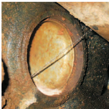
RUST ATTACKS PARTS FROM THE INSIDE OUT in a very big way. It clogs radiators and can erode an expansion plug that, on the outside, looks just fine. We replaced all the expansion plugs in a 1998 Taurus while we had the transmission out and washed enough rust out of the block to fill a large coffee can. And it wasn't even overheating.
