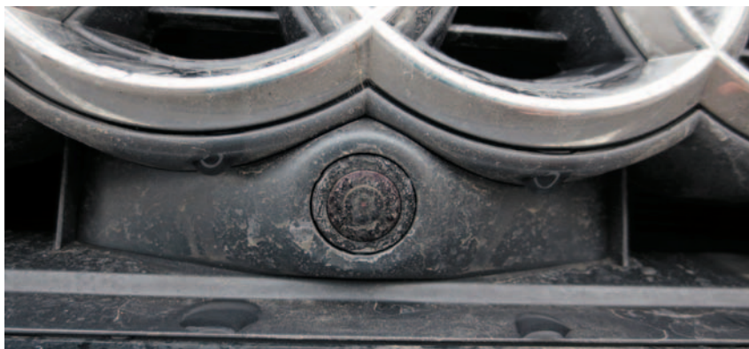
SALT AND ROAD GRIME is covering the forward camera. Clearing it off is a nice professional touch.
