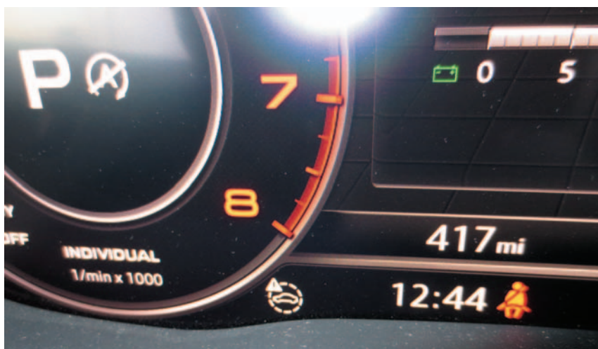
THE TINY WARNING LIGHT on this 2017 Audi A4 Quattro indicates a problem in the forward warning system — part of the pre-collision system. It's worth having a quick look around before sending this off to the dealer for repair since it might be a simple fix.
