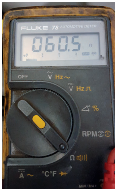
TERMINATION RESISTANCE was tested on the Corolla and no faults were indicated.
