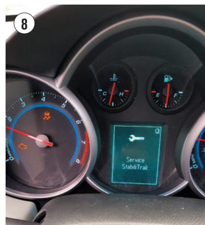
2012 CHEVROLET MALIBU with a StabiliTrak warning message on the dash. This vehicle didn't actually have a stability control problem.
