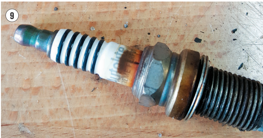
HERE'S THE CAUSE of our Stabilitrak light on the 2012 Malibu (seen in Fig. 8).
