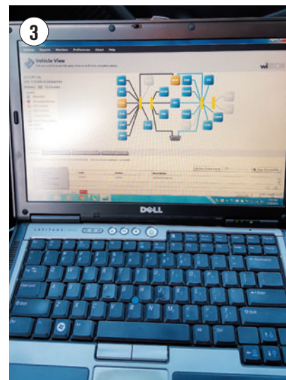
USING THE Chrysler Wi-Tech to see what modules are communicating. Anything in yellow has an issue.
