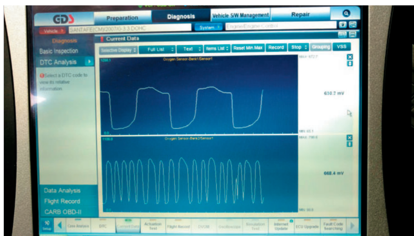
THE DATA obviously matches the code description for a slow responding Bank 1 O 2 sensor, but the graph of the sensor looks eerily familiar to a post cat O 2 sensor.
