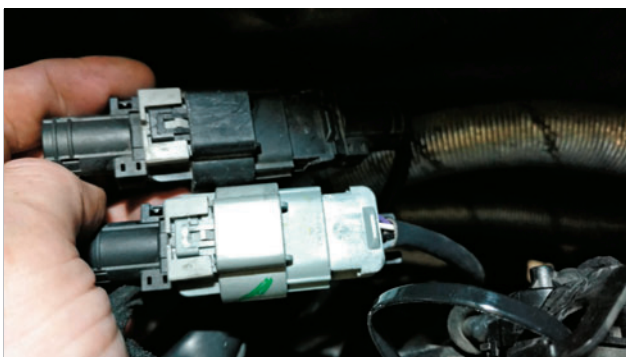
THE BANK 1 FRONT and Bank 1 Rear O 2 sensors are located right next to each other in the darkness of the back of the intake plenum and the firewall.
