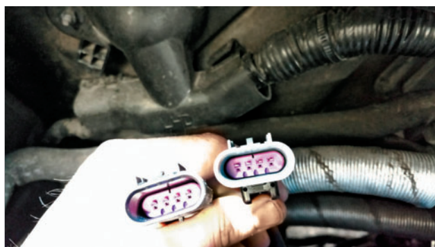
NOTICE THAT WITH THE FRONT and rear oxygen sensor connectors unplugged, the locating tabs are identical so the technician did not notice any problem with reconnecting them in reverse locations.
