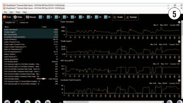
SCAN DATA GRAPH SHOWING the change to EIVC mode and manifold pressure remaining high at light load
