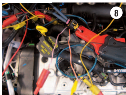
PICTURE OF THE SETUP with jumper wires installed for the circuit resistance experiment
