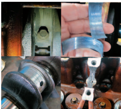
THIS IS WHAT HAPPENS when you keep driving after all the oil has found a new home. It's interesting that only one rod burned out — the others didn't suffer at all.
