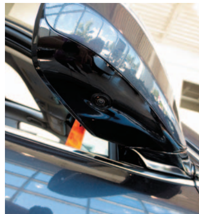
SENSORS FOR BLIND SPOT DETECTION SYSTEMS are typically located on the bottom of the side mirrors.
