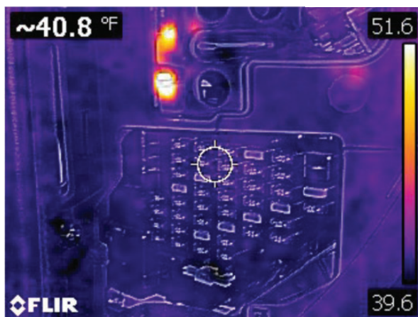
FUSE BLOCK WITH no current draw (C2 Camera with MSX)
