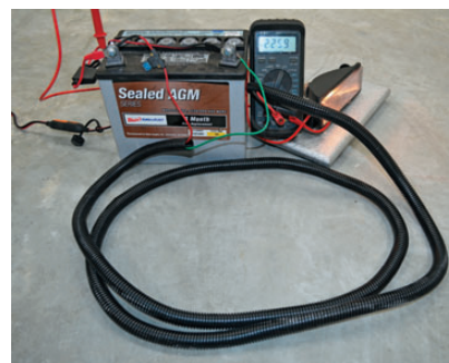
SIMULATED HIGH RESISTANCE light circuit with 2.25V Drop in 6' harness
