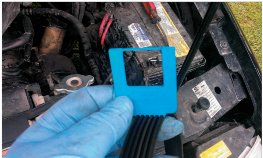
To check a serpentine belt for wear today requires a special tool like this one made by Dayco.
