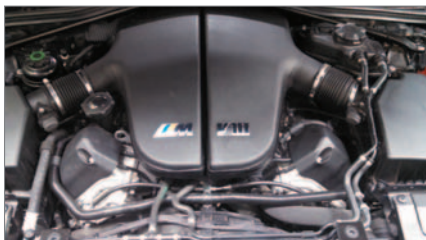
The Throttle-Valve Actuators are hidden under the air intake plenum. Each of the throttle bodies have individual air boots that need to be loosened to remove the air plenum assembly.
