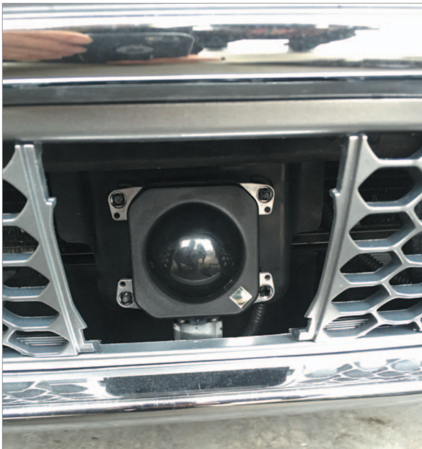
A minor fender bender took out this expensive radar module, and installing it is only half of the job.
