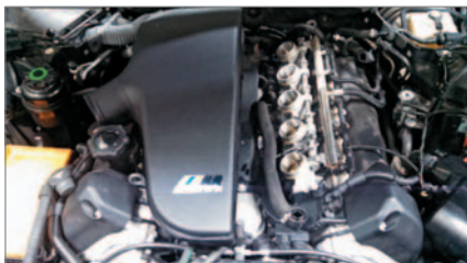
The Throttle-Valve Actuators are hidden under the air intake plenum. Each of the throttle bodies have individual air boots that need to be loosened to remove the air plenum assembly.
