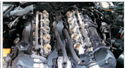
The Throttle-Valve Actuators are hidden under the air intake plenum. Each of the throttle bodies have individual air boots that need to be loosened to remove the air plenum assembly.
