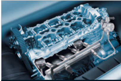
Increasingly popular as a way to boost fuel economy, GDI places the injector directly in the combustion chamber.
