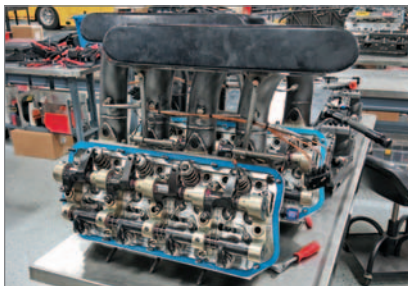
With the level of competition in the NHRA, every run has to start with a peak engine. That means, in part, heads are changed after every run with new ones. Clutches are also changed after every run.
