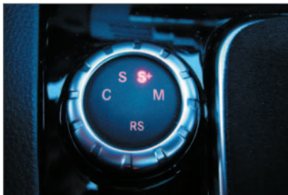
The shifting selector on a Mercedes AMG C63 with a Speedshift MCT (Multi-Clutch Technology) 7-speed transmission. When in the Sport Plus and Manual modes, gear changes occur at a lightning fast 100ms between shifts.
