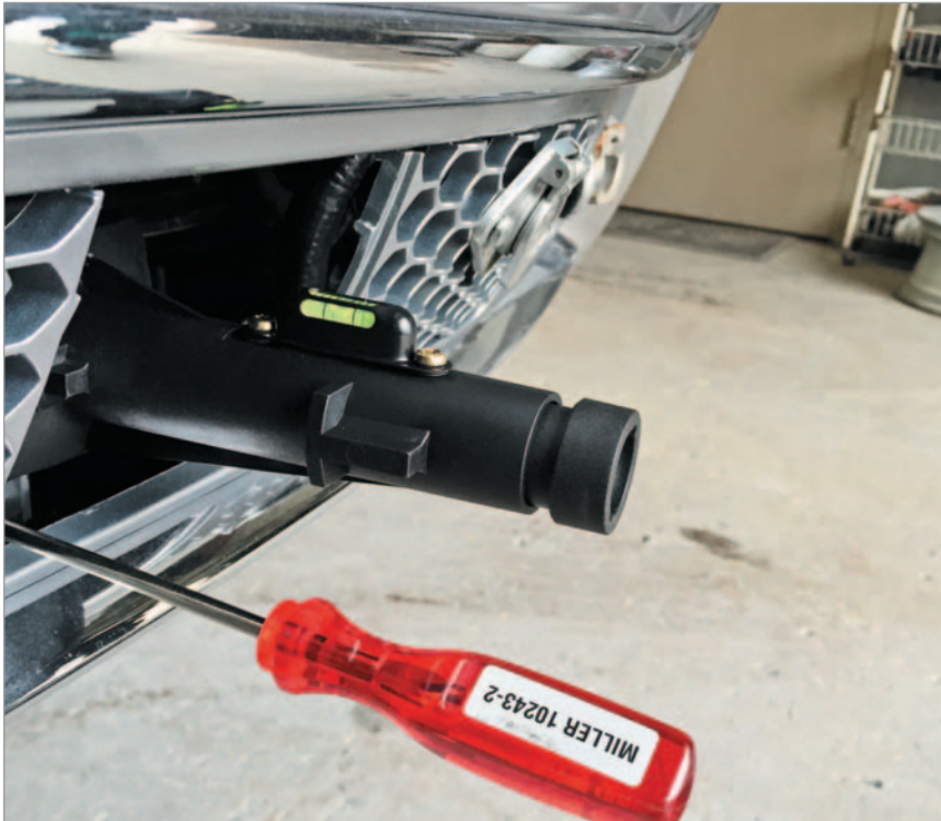
During the vertical calibration procedure, this tool levels the radar head to the surface.
