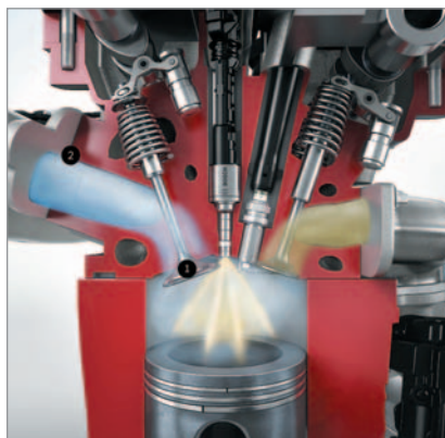
GDI engines typically build carbon on the back of the intake valve and along the intake runner.
