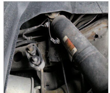
Note connectors for rear unit. There is a different pigtail configuration for the front units.
