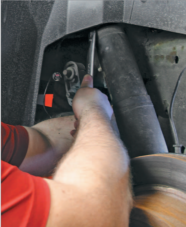
Removing rear unit. Ensure axle is properly supported before removing upper and lower mounting bolts.
