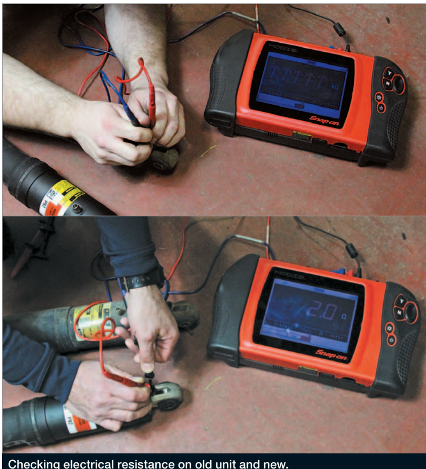
Note connectors for rear unit. There is a different pigtail configuration for the front units.
