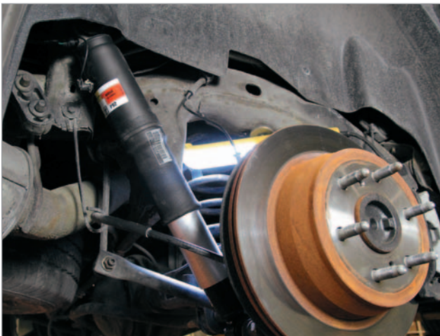
Installation completed. Before driving, ensure air compressor has inflated the shock's air boot.
