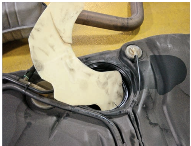
One lesson I learned the hard way on a Saab repair — this broken tank baffle was the cause of an erratic fuel gauge.
