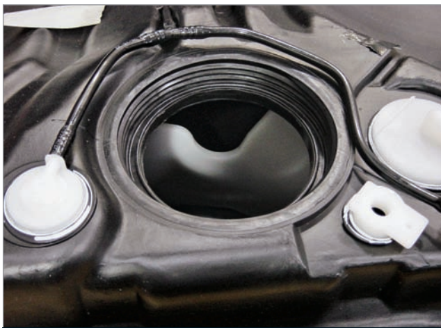
The baffle in place on the replacement tank. Below is an indentation that must line up with the pump on install to prevent the sending unit from hanging high.
