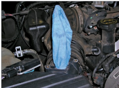
2004 Ford Explorer 4.0 litre restriction in air intake system
