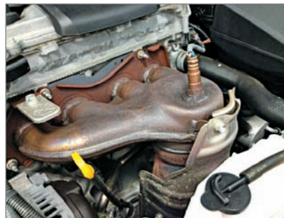
AF sensors may look identical to their O 2 sensor counterparts but they function much differently.
