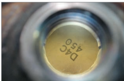
Case study vehicle — internal boroscope view of new catalyst substrate.
