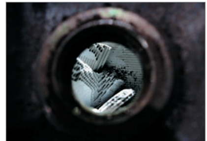
Case study vehicle — internal boroscope view of the damaged catalyst substrate.
