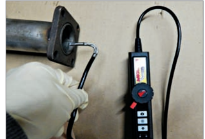
Boroscope being used for proper diagnosis and verification.
