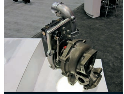
The Garrett turbocharger used on the EcoDiesel has a rotary electric actuator (REA) to control the variable nozzle.
