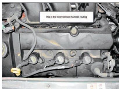
This is how the wire harness looks when installed incorrectly.
