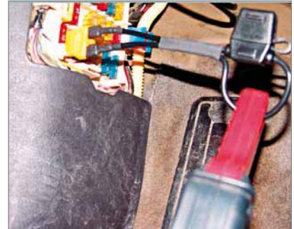
The fuse loop is inserted into the fuse 15 cavity. The low amp current probe is hooked to the fuse loop so any amperage change on the circuit can be recorded on the lab scope.
