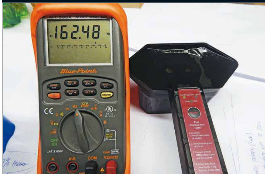
This is a pure alcohol reading on the Kent Moore tester.
