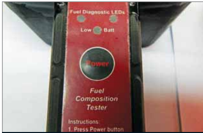
Turn the tester "on" after adding the fuel sample to the test tray.
