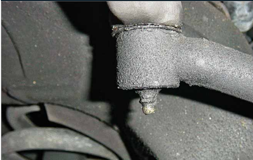
If the suspension/steering system is fitted with lube points, take a minute or two to wipe them down and grease them up.
