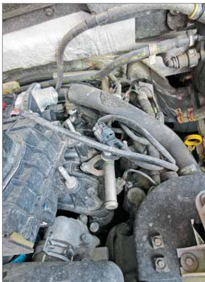
Note the sensor on the fuel rail rather than a regulator in the 2007 F-150 returnless fuel system.
