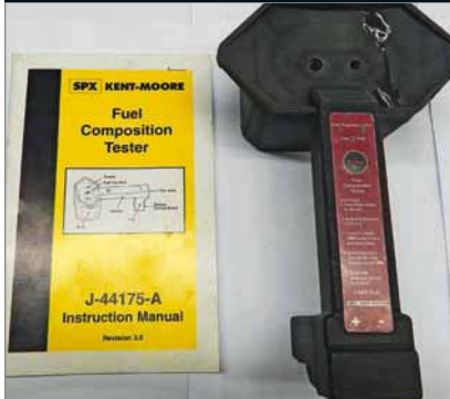
This is an older Kent Moore fuel composition tester I use for checking fuel samples.
