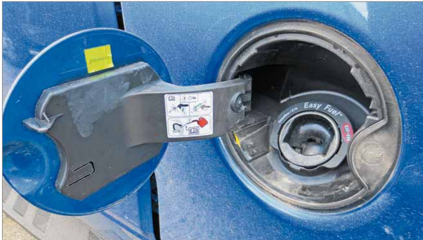
This 2012 Ford Raptor doesn't have a fuel cap, the 2007 F150 does. Either way, it's really important to keep the area clean so dirt doesn't end up in the tank or the fuel rail.
