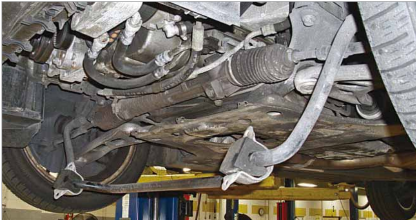
Believe it or not, that's the way I found this BMW. The sway bar nearly hit me in the head after I removed the undercar panel.
