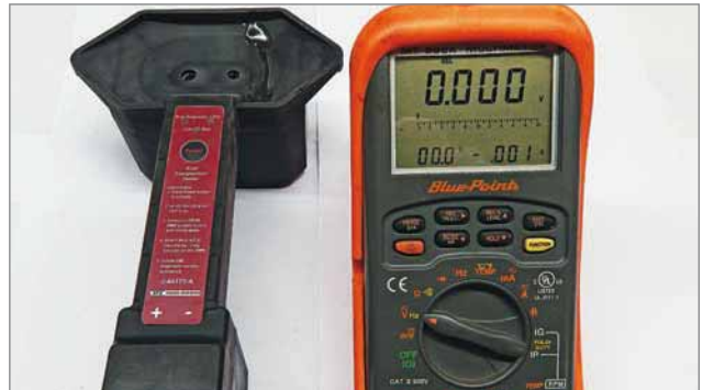
Connect your DVOM to the Kent Moore tester and select the frequency function, measuring in Hz.
