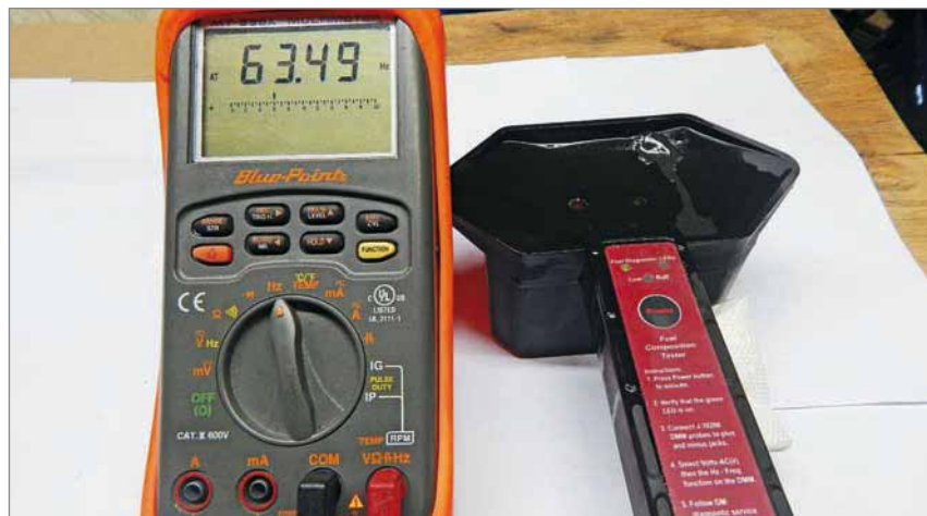
Take 50Hz off of the meter reading to get alcohol percentage. In this case, a little over 13 percent.
