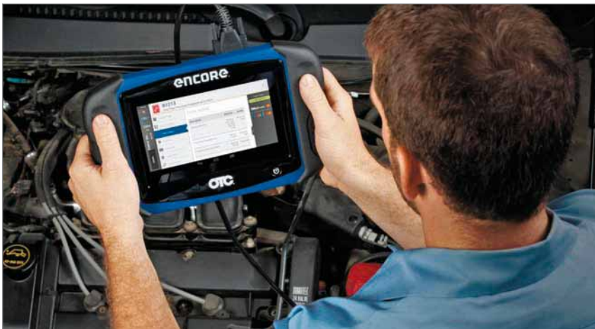
The OTC Encore is the company's first tablet scan tool. It is on the Android platform.
