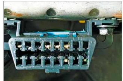
This DLC has been mangled by improper testing.
