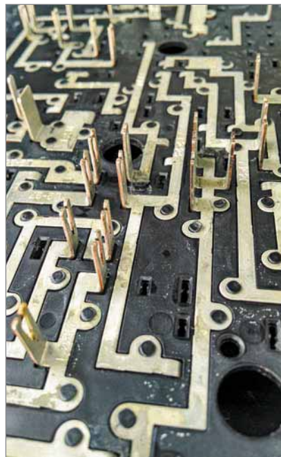
This GM UHFB had severe corrosion.
