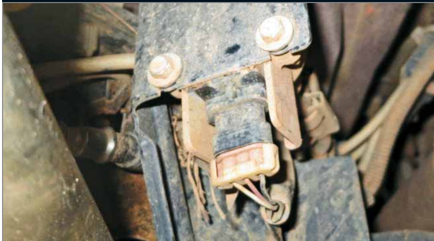
When we finally duplicated the no-start and discovered the spark plugs were wet (which would be an overfueling issue due to false data from this FCS), we also discovered that we could floorboard the accelerator to put it in clear flood mode, drying the plugs so it would start.
