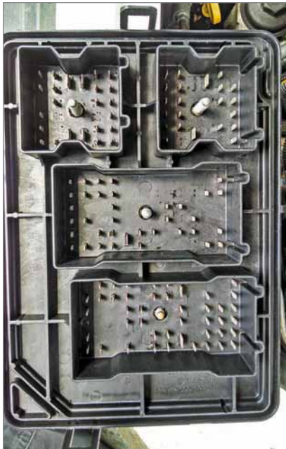
Windshield or coolant leaks or battery fumes can lead to problems.
