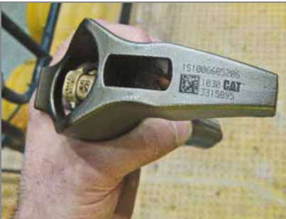
The serial number of the injector is used to find its trim file, which is calibration software for that specific injector.
