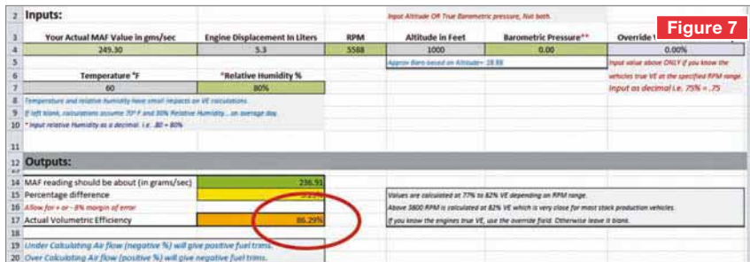
Results of a volumetric efficiency calculator using the MAF data as a tool to verify the MAF is reporting properly.
