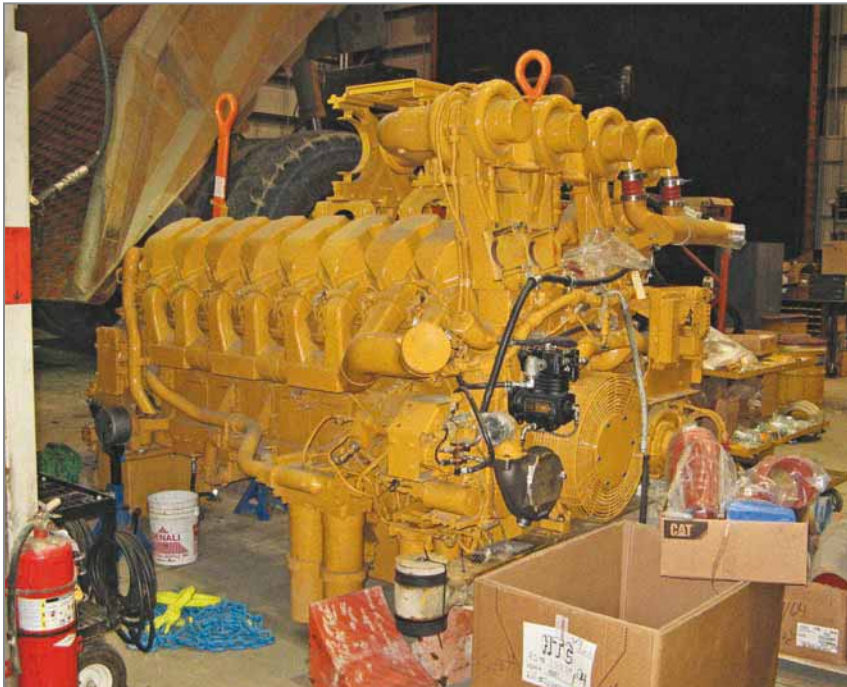
The 793F is powered by a 16-cylinder version of the C175 diesel engine. This engine produces 2650 horsepower and meets EPA Tier II emission standards.
