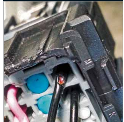
Damage that looks minor, like this Nissan TCM wiring, can cause voltage drop, and resulting circuit malfunctions
