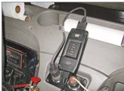
A communications adapter is used to connect a laptop computer's USB port to the nine-pin data link.
