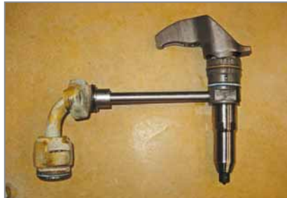
The HPCR injector and quill tube used in a Caterpillar C175. The quill tube makes metal-to-metal contact with the body of the injector.
