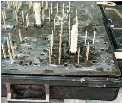
Corrosion caused plate layers to warp.
