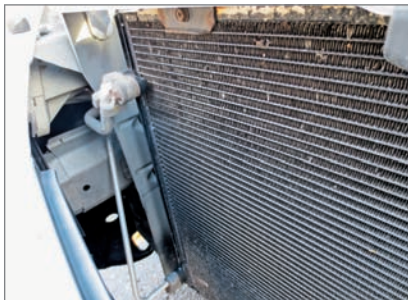
Common locations for leaks on AC condensers, at the lower corners (both at the front and on the inside by the rad) and at the connections (especially ones exposed to the elements).
