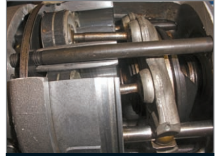
These two photos of a cutaway CVC show high displacement (top) and low displacement (bottom).
