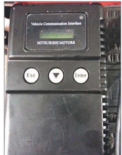
MUT III is a PC-based scan tool that uses a Vehicle Communications Interface (VCI), shown here.
