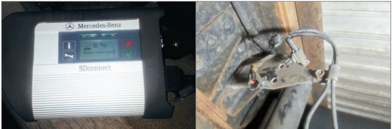
(Left) A phone call to a Mitsubishi tech friend answered my communications questions, and I found out that my MB scan tool VCI would do the trick. (Right) After verifying the circuit path between the sensor and the module was intact, the only thing left was the sensor itself. But I still want to confirm that's all it is.
