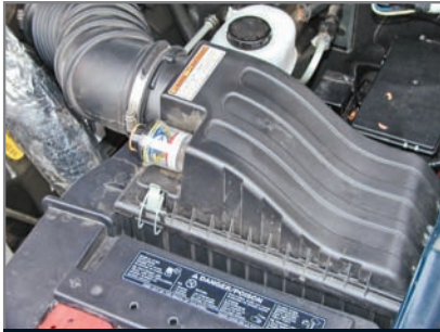
This is an early model air cleaner on a 7.3L with the Filter Minder gauge.
