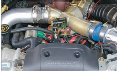
This is a late model 7.3L with the glow pug module. It is the silver box with the light green and black connectors.
