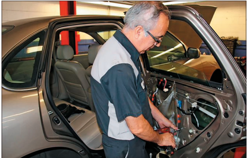
Technician Emilio Chavez replaces a passenger rear window regulator on a 1998 Toyota Avalon for a customer.
